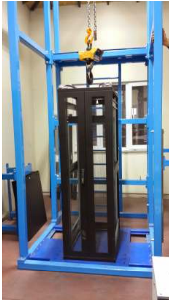
Photo 11 - The test cabinet bolted to the floor
