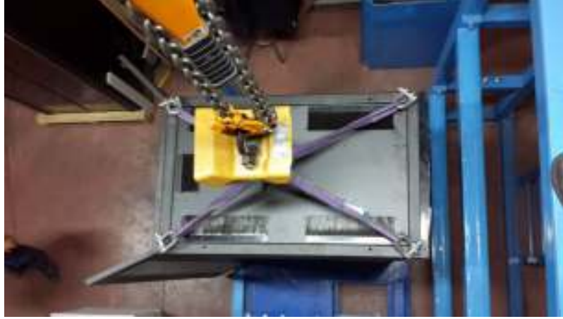
Photo 13 - The test cabinet lifting points
