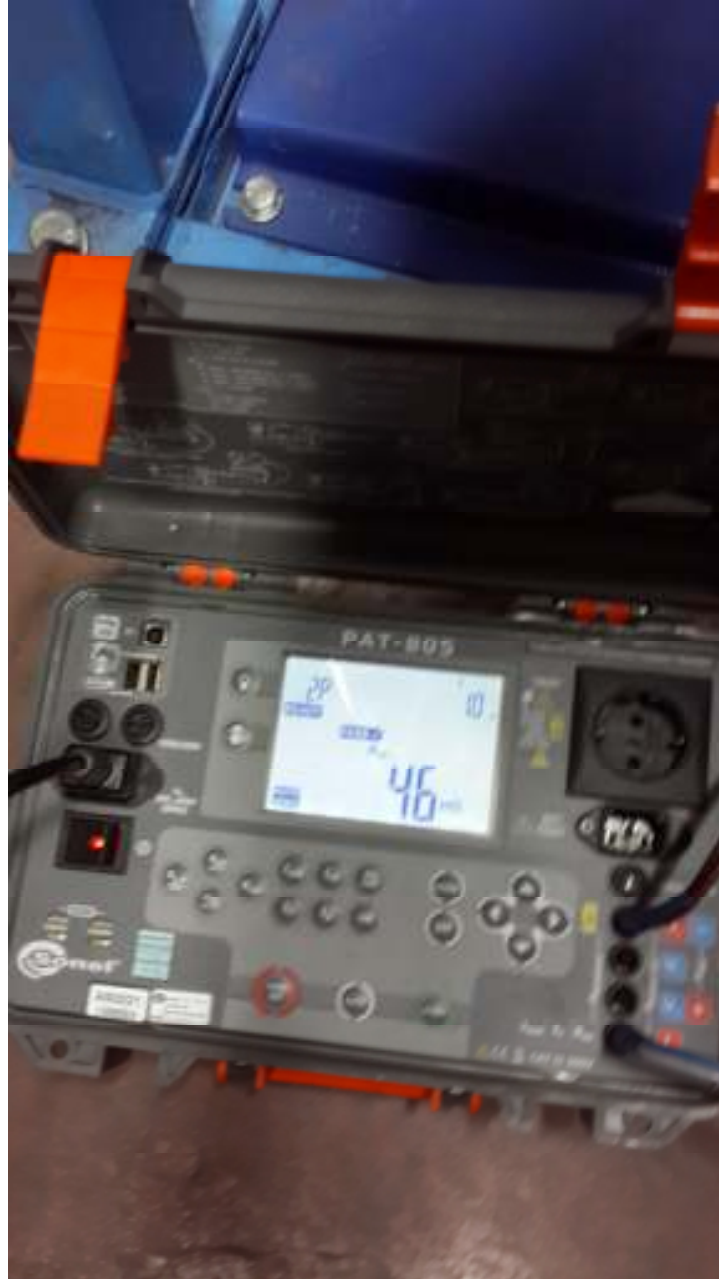
Photo 15 - The test cabinet earth bond continuity test
