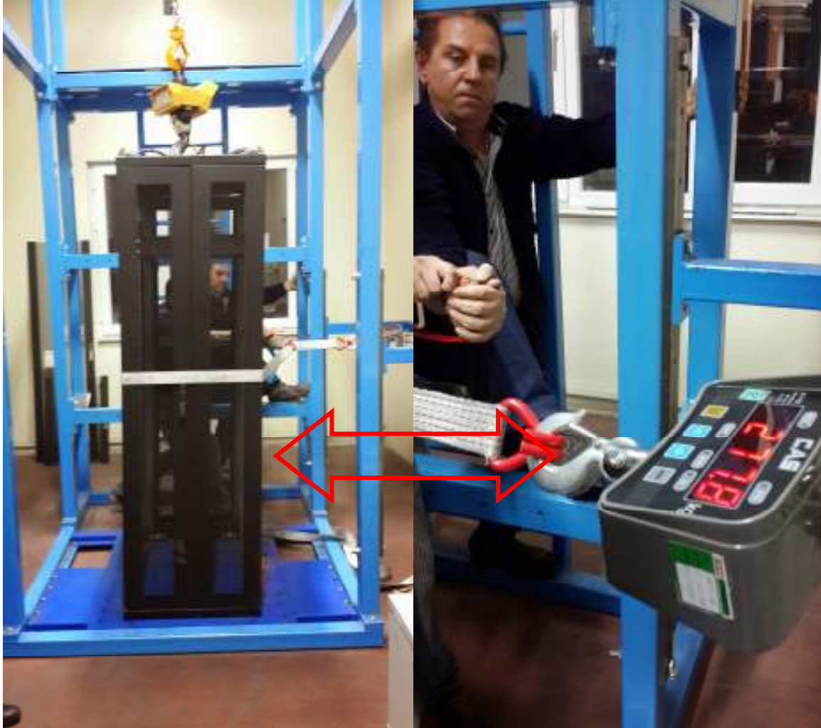
Photo 17 - The test cabinet applied the force
