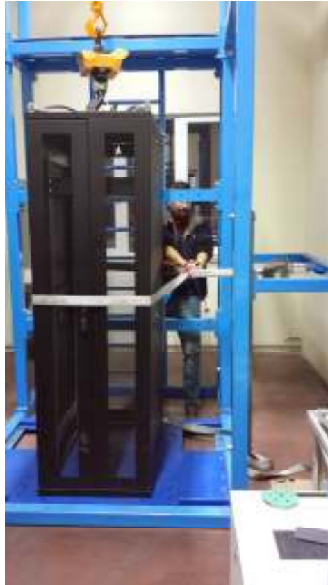
Photo 16 - The test cabinet bolted to the floor
